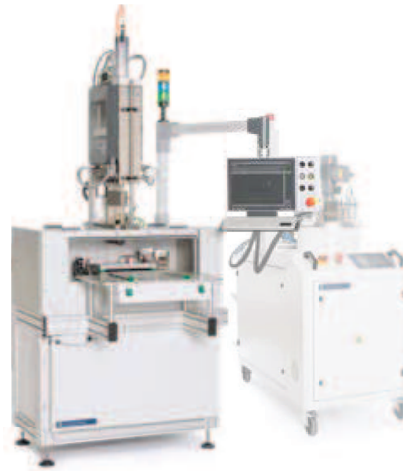
VDS P with Dos P-X dispenser, 2 component, 4 nozzles; A310 60/20 preparation and feeding unit, 2 component
