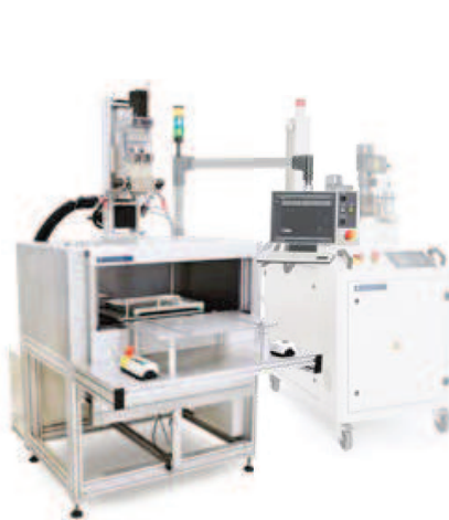
VDS U with Dos P050 dispenser, 2 component, 1 nozzle; A310 60/20 preparation and feeding unit, 2 component
