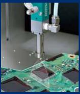
Spot coating by non contact high speed jet.
