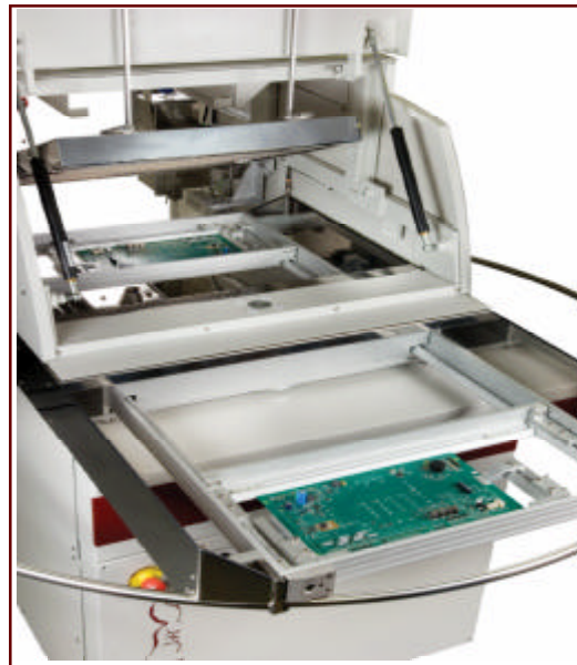
Jade-Handex adjustable tooling rotate mechanism.
