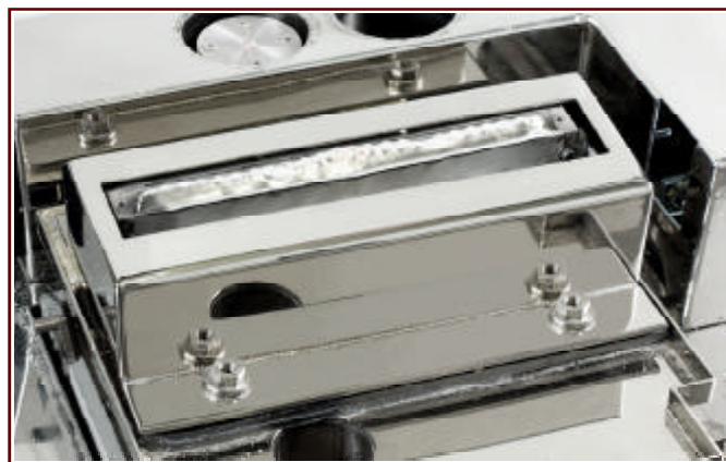
Optional 150mm wide wave solder nozzle and nitrogen shroud.
