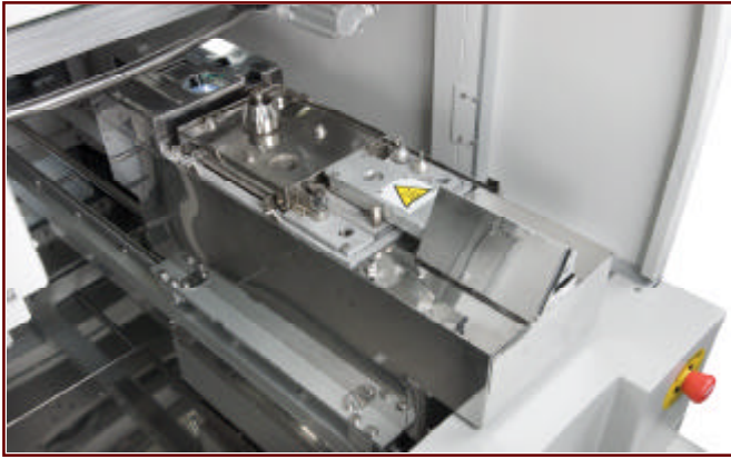
Solder nozzle, nitrogen shroud, Drop-Jet fluxer and programming camera assembly
